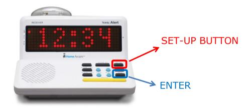
4. Press and hold down the link button on the bottom of the HA360VPT. The red light on the transmitter will light up. Release the button and the words PICK A DEVICE will begin to scroll on the display of the main
